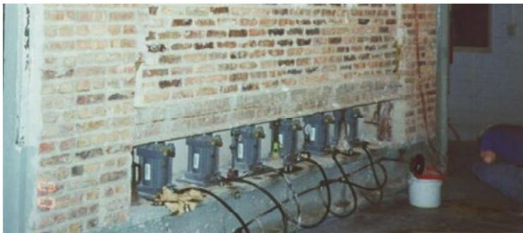
ASTM E119 Test Assembly, Exterior Side
