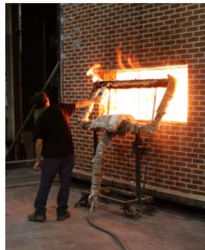
Figure 4: Fire emitting from the test window
