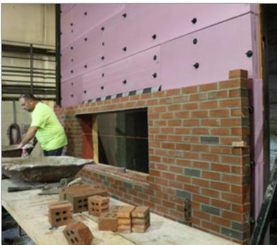
Figure 3: FOAMULAR® NGX™ test wall under construction
