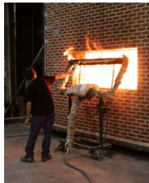
Figure 4: Fire emitting from the test window
