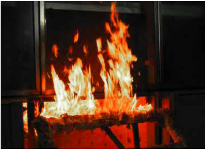
ASTM E2307 room and exterior window burner fire exposure.
