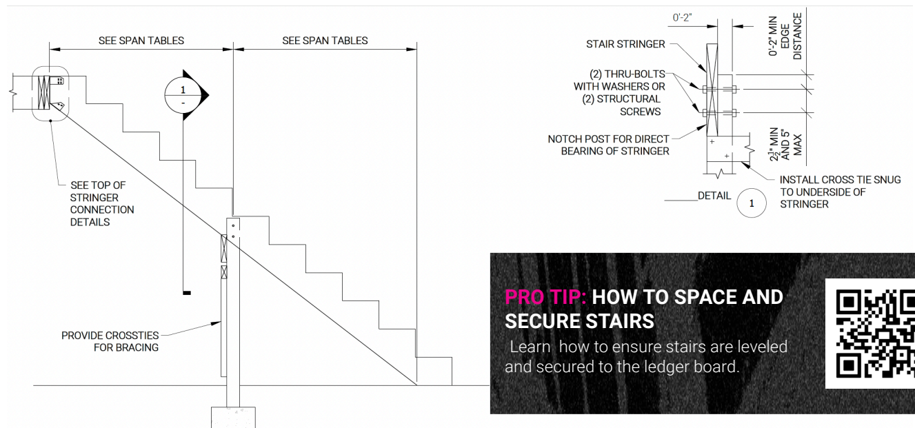
Figure 3: Mid-Span Support Detail
