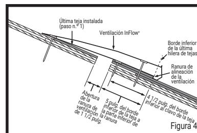
**Step 7:** Using the nails provided, hand-nail the InFlow® Vent in place using the built-in nail holes. Continue installing vents flush with each other from rake edge to rake edge. When installing the final vent, cut the non-rake edge of the vent (if necessary), to ensure a factory-finished edge is flush with the rake edge.
