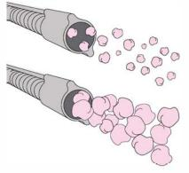
Different density settings when in attic mode to ensure tight attic spaces are adequately and easily insulated.
