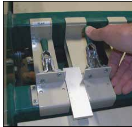
Figure 2 – Spacing with a gage block
