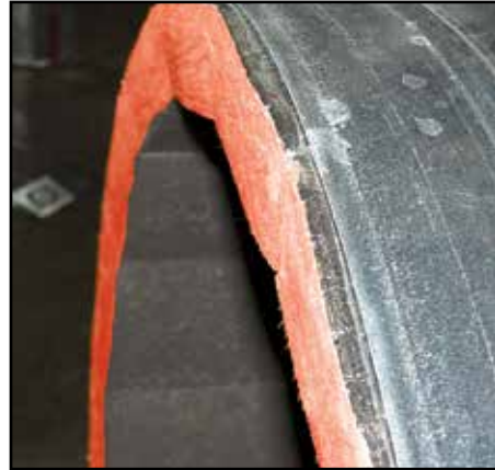
Figure 14 - \frac{1}{8} " additional liner on couplings and fittings
