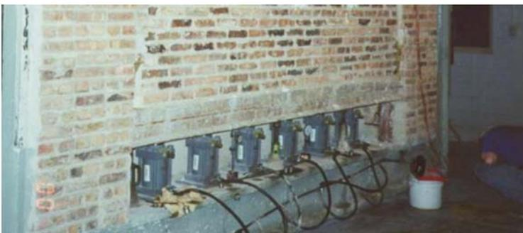
ASTM E119 Test Assembly, Exterior Side
