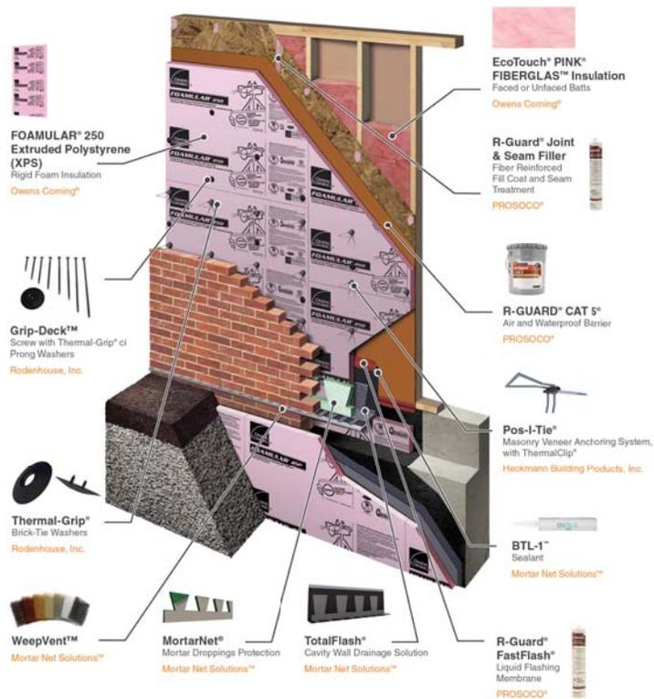
The CavityComplete® Wood Stud Wall System excludes the masonry veneer, wood studs, interior gypsum board and exterior sheathing. A detailed list of the components is available at [www.CavityComplete.com](http://www.CavityComplete.com).
