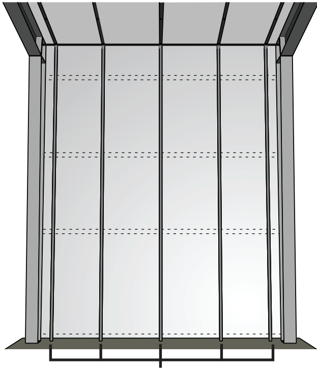
WALL BANDING MATCHES ROOF BANDING PATTERN
