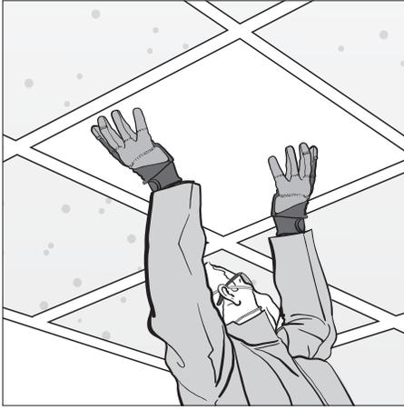
**Lower** ceiling tile and overlay onto the grid for a fresh new look
