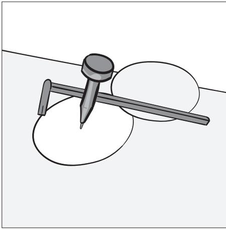
**For lighting/ventilation/sprinkler integration,** cut the ceiling overlay at the right dimensions with a cutter or appropriate cutting machine.
