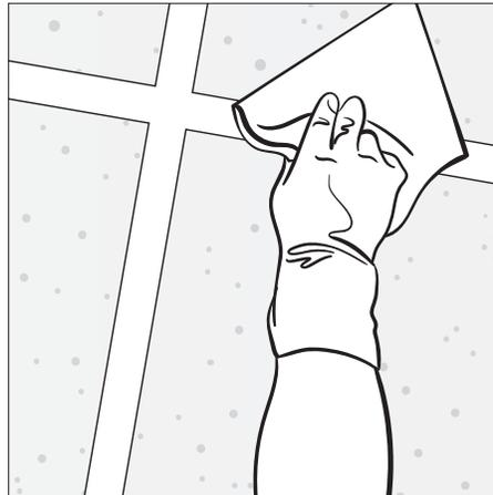
**Clean/degrease** the grids before renovation tile installation\*.
