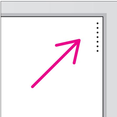
**Identify the installation direction** of the Bright & Up™ overlay tile based upon the location of the holes.
