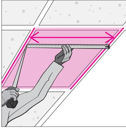
**At room edges:** measure length and width at center distance **and allow 10mm more** to compensate the acceptable sagging of the overlay (5-6mm per 600mm).
