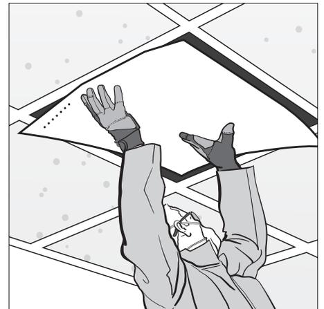
**Position** the Bright & Up™ ceiling overlay tile, smooth side down, directly beneath the existing tile.
