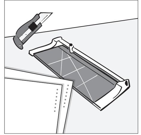
**Cut** the ceiling overlay with a cutter or a paper cutting machine for a cleaner cut. Up to two tiles can be cut at the same time.
