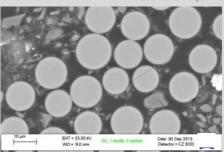
This is a cross-sectional view of a Slurry-FIL™ bundle that is completely encapsulated within the slurry surfacing matrix. This tight fiber configuration guaranties the fiber strands will perform as intended.
