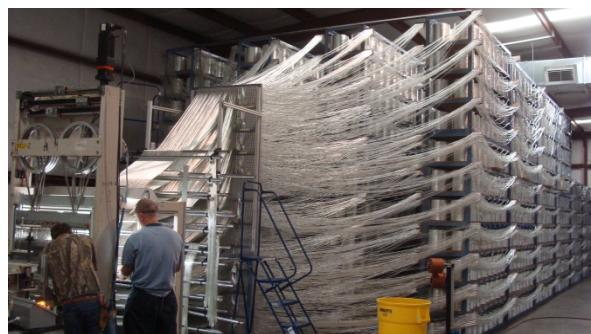
scaled-up 3D woven fabrics made with Advantex® corrosion-resistant glass. Advantex® glass fiber reinforcement is a patented boron-free glass formulation that is both a corrosion-resistant E-CR glass fiber reinforcement meeting ASTM Standard D 578 and
